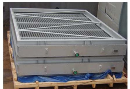
FINNED TUBE TYPE HEAT EXCHANGER
